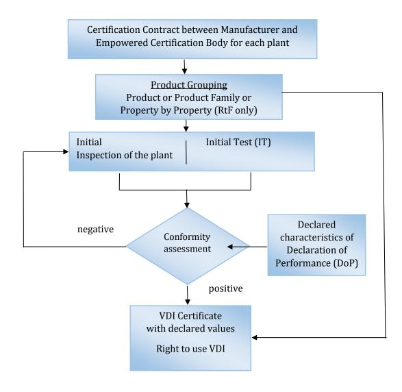
Figure 1: The Certifiction System (Initial Testing)
