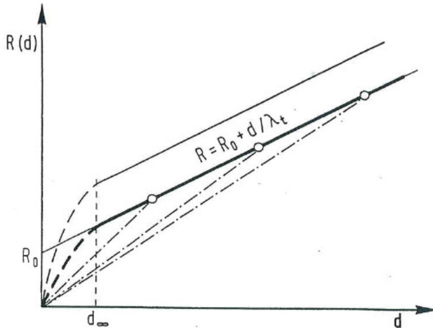
The thickness  $d_{\infty}$  indicates the beginning of the straight portion of the plot of thermal resistance,  $R$ . A reduction of apparatus emissivity shifts the bold line upwards.
