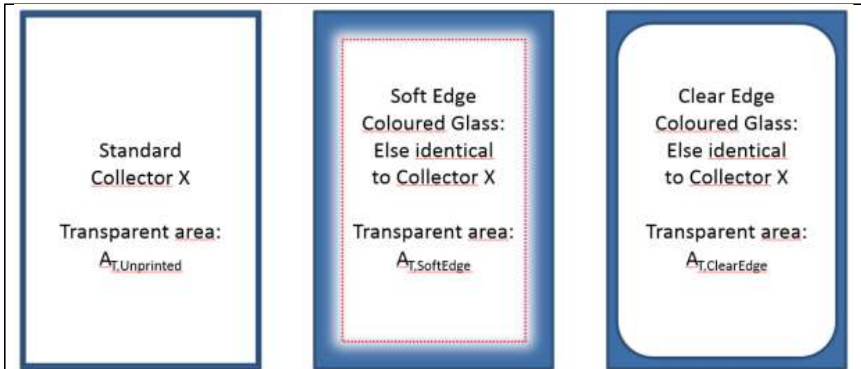
Figure 1, Edge Printing: Left: unprinted. Middle and right: typical examples of edge coloured glasses
