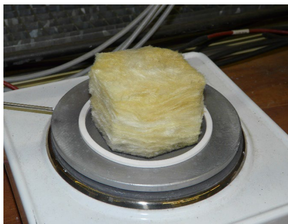
Figure 3: Test sample placed on the aluminium disc. The black fleece is placed on the heating plate to simulate direct contact with a hot absorber.
